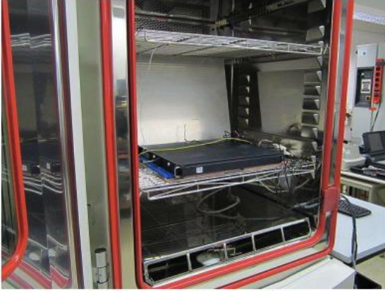
Fig. 12: Device in Climatic Chamber
