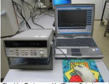
Fig. 11: Test assembly (Temp.-Data-Logger)
